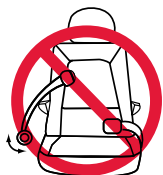
Lap belts with a sewn-in latching mechanism that have a retractor that locks only in case of a sudden stop.
